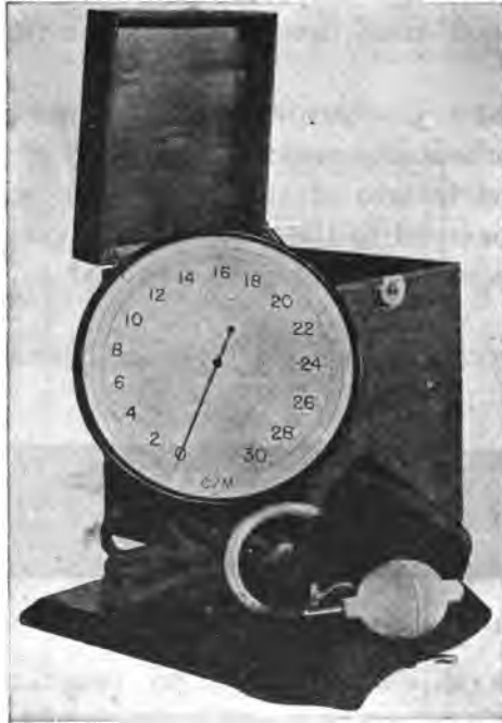
Fig. 34.—Sphygmomanometer with a dial 8 inches in diameter and may be read across a room. This large dial magnifies the oscillations of the needle. The range is 300 mm. The dial is adjustable to any position.
